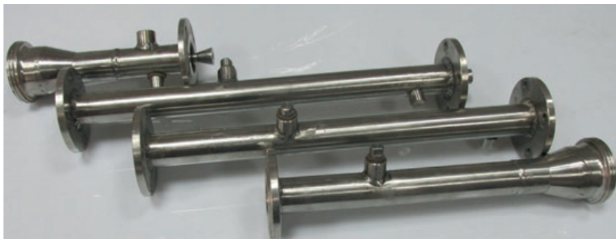
Fig. 1. Experimental samples of cavitation devices
