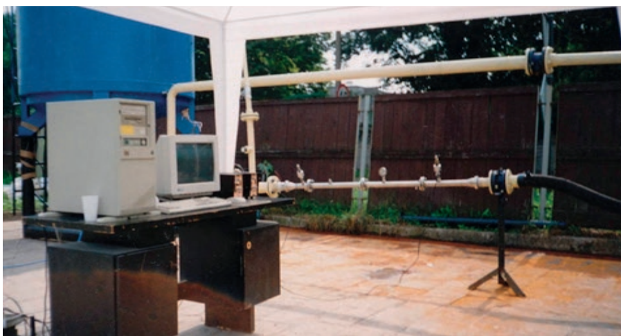
Fig. 2. Experimental stand for hydrodynamic cavitation
