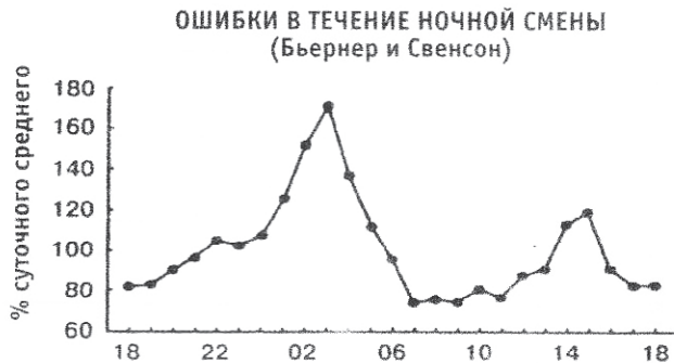
Fig. 1 - Errors as a percentage of the daily average, made the night workers (N = 62000) that perform different types of visual works for various night shifts (adapted Kerhofom).
